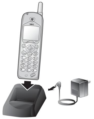
To recharge a handset (with the battery pack inside) place phone here.
